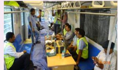
Sandbags loaded for Conducting Oscillation trials in AW4 load Condition
