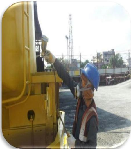
Nose mask with cartridge using for painting and spraying of paint for vehicles.
