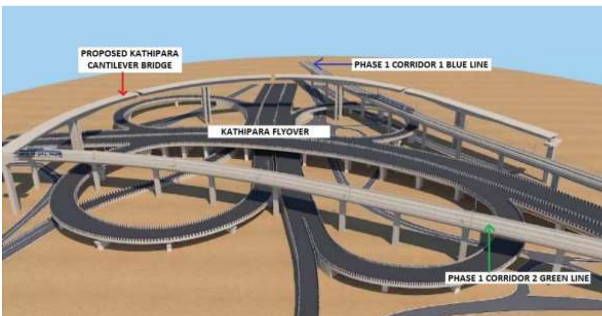
Fig. 3.9: Concept diagram of intersections between Proposed Kathipara GS and existing infrastructures
