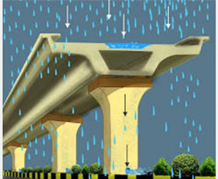
Concept Diagram - Rain Water Harvesting in Metro Via-
